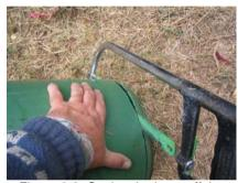
Figure 6-8: Cutting the base off the bucket
