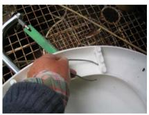
Figure 6-15: Using a hot wire to make a hole through the plastic toilet seat ribs
