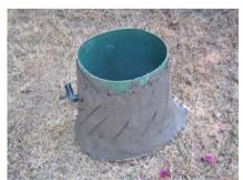
Figure 6-21: Upper-half of bucket covered in concrete
